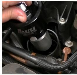
**Step 4:** Lubricate the 1/8" hex plug and install in unused port.
