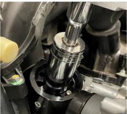
**Helpful Hint:** 90-degree fitting can be installed using a 15/16" 12 point closed end wrench.
