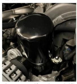
**Servicing instructions at Oil Change:** Prior to draining engine oil from oil pan, and oil filter removal, remove oil filler cap and apply minimum 30 PSI to the Schrader valve for at least three seconds. This will evacuate the oil retained in the oil filter and cooler. Then, remove oil filter and replace.
