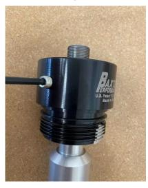
**Step 5:** Install tip and body O-ring seals and lubricate with engine oil. (Verify Face seal is in place)
