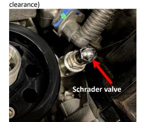
**Step 8:** Lubricate threads on Schrader
