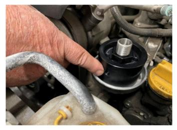
**Step 4:** Remove adapter. Apply oil to hex plugs and install in two ports not utilized. (If using sealing tape, be sure tape is on treads only and not end of plug)
