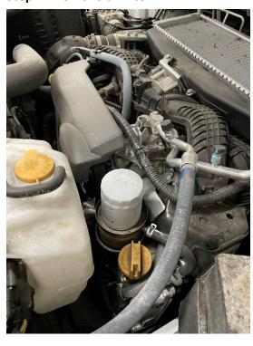
**Step 2:** Install adapter without base seal O-ring. Torque to 30 ft. lbs. using 1" Deep Socket.
