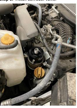
**Step 7:** Install an appropriate size oil filter that contains M20x1.5 threads. Subaru oil filters will fit this adapter. **Caution:** Make certain that filter/adapter height will not contact hood when closed.
