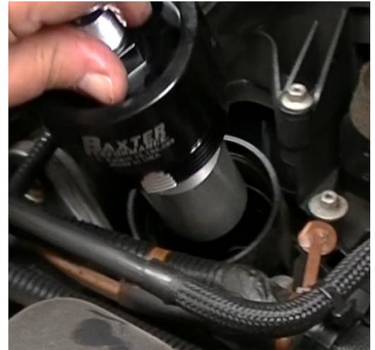
**Step 5:** Install tip and body O-ring seals and lubricate with engine oil. (Verify Face seal is in place)
