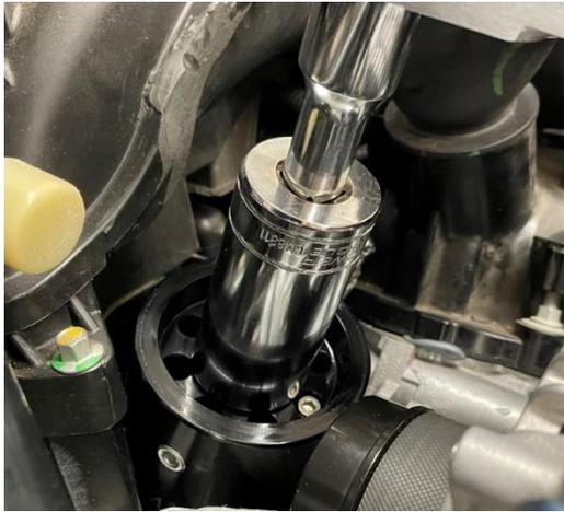
**Step 7:** Lock the adapter in place, by tightening the socket head cap screw with a 5/32 hex wrench.
